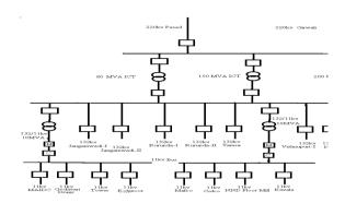
fig 6. Single line diagram for substation 220KVA
