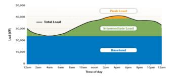
fig 4.. for supply and demand load curve
